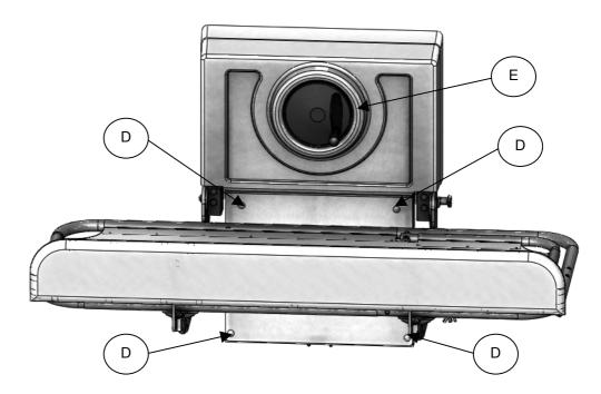
• Fit the hand wheel (E) to the spindle and secure in place with a M8 x 16, and 1 x M8 flat washer. Operate the hand wheel to ensure the shower stretcher raises and lowers satisfactorily. Press in place the plastic dust cap.
