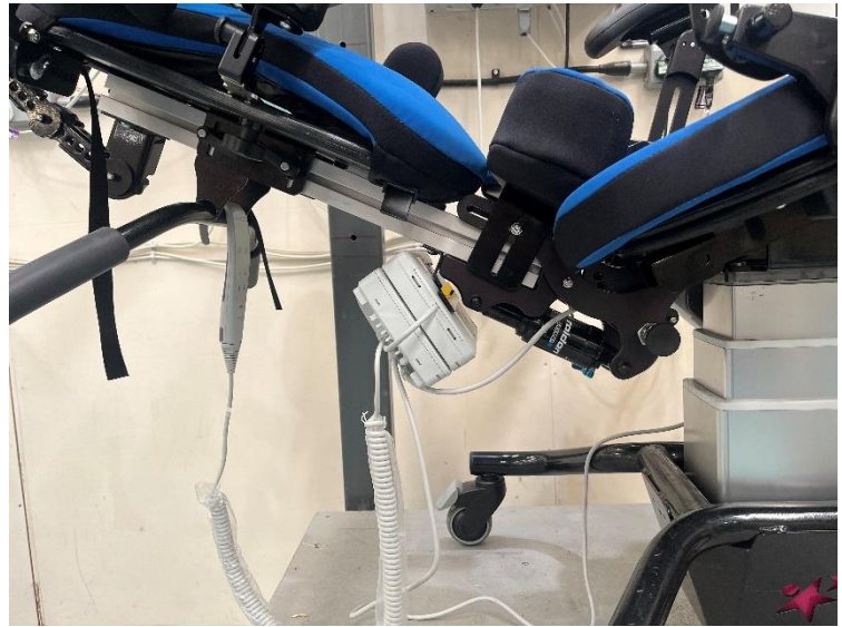
Backrest static load test images
