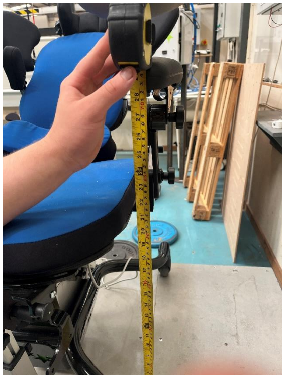
Leg rest (+ split leg design) static load pre-test measurements
