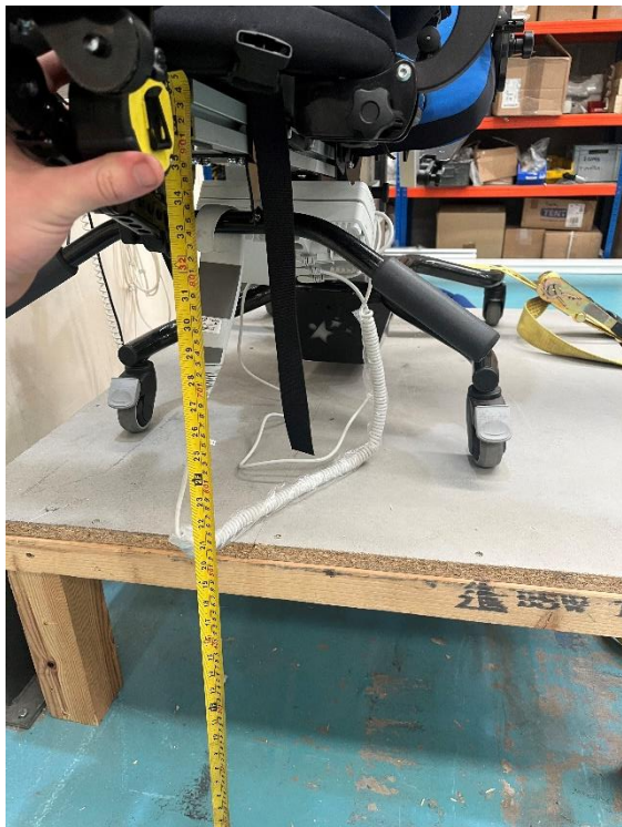
Arm rest static load under load measurements
