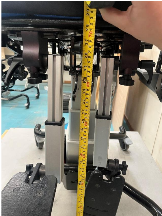
Backrest static load pre test measurements
