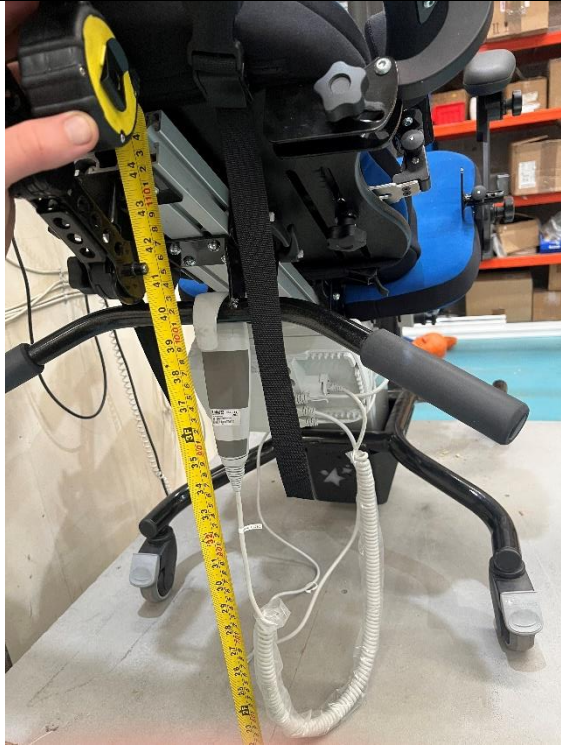
Armrest static load pre test static load measurements
