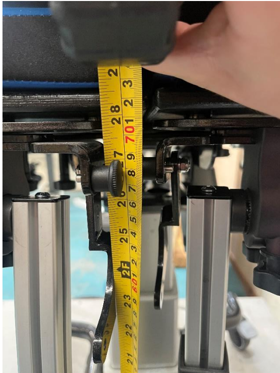
Seat Static Load Pre Test measurements
