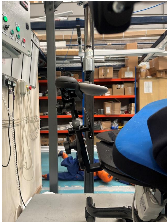
Leg rest (+ split seat design) static load test images
