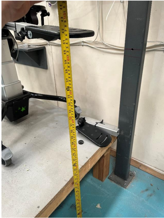
Leg rest (+ split seat design) static load post test measurements
