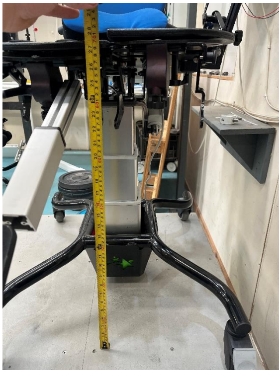
Leg rest (+ split seat design) static load under load measurements
