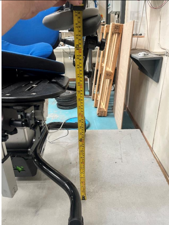
Leg rest (+ split seat design) static load under load measurements
